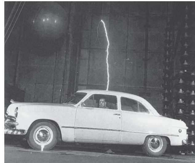
Figure 24-22 A large spark jumps to a car's body and then exits by moving across the insulating left front tire (note the flash there), leaving the person inside unharmed.
